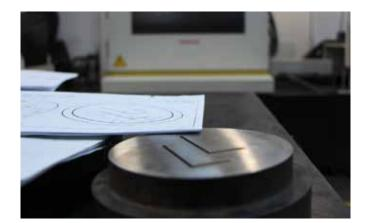
In this industry, accuracy is a must when creating a die, because even the smallest error when gone unnoticed, can cause a significant amount of products to become defected, therefore the 0,001mm precision that is offered by ROBOCUT is highly valued in this process. The machine is running 24/7 since its installation four years ago, in three shifts, producing approximately 9-10 dies a day.
